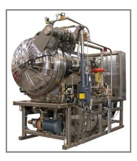
The research and development retort and the expertise of the laboratory personnel enable development work to be done outside of a food processor's facility. This eliminates the loss of production time that would result from
