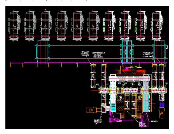
The retorts are configured with the required front-end and back-end consolidating machinery that is specific to the package. A pouch loader/unloader, a can loader/unloader, a tray loader/unloader, etc., are designed to feed into, and pull from, the retort line.
