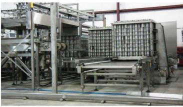
Speed, throughput, labor savings, and reduction in lost-time due to injury are the hallmarks of these retort room automation systems – shuttle transfer and retort loading (left) and automated basket loading (right.)
