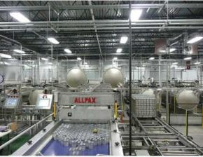
Empty baskets (left) are automatically indexed to a can accumulation and basket loading system (right.)
